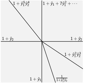
A scattering diagram is a set of walls. Each wall is a codimension-1 cone in  $V^*$ , decorated with a scattering term—a formal power series in the  $\hat{y_i}$ .
